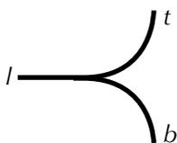
A train entering a point along one of the curved pieces of track must exit along the straight portion; i.e. a train entering from *t* or *b* will exit via *l*. A train entering via *l* will exit via *t* or *b* depending on the point.
